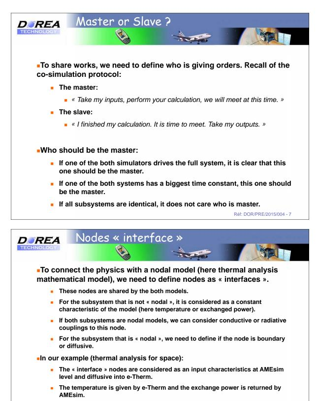
In our case (heat transfer), the exchange power of interface nodes are considered as internal powers within the equation.
