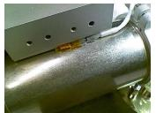
Temperature sensor of one motor housing
