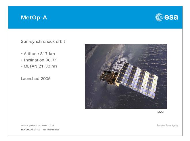
MetOp-A has an orbit typical of sun-synchronous earth observation satellites. It was launched in 2006 so here the real spacecraft position data for the period 2007-2011 could be imported into the simulation. This allows us to observe the actual features/weather the spacecraft flew over.
