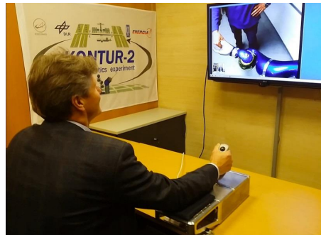
Cosmonaut handshake training with the KONTUR-2 joystick engineering model and the DLR humanoid robot Justin between the cosmonauts G. Padalka and O. Kononenko
