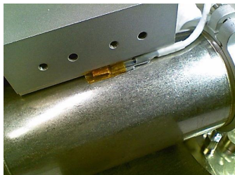
Temperature sensor of one motor housing
