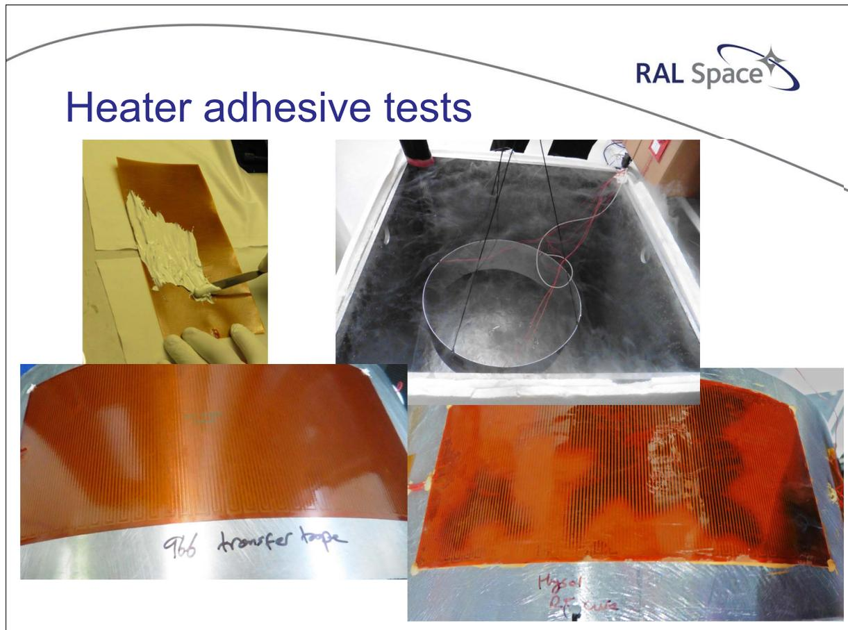
As I said earlier, I've used thermal analysis to size the power requirements and also the locations of the heaters on the blackbody. But in reality, ensuring the heaters maintain a good thermal contact with the structure is down to the adhesive working across the range of operational temperatures.
