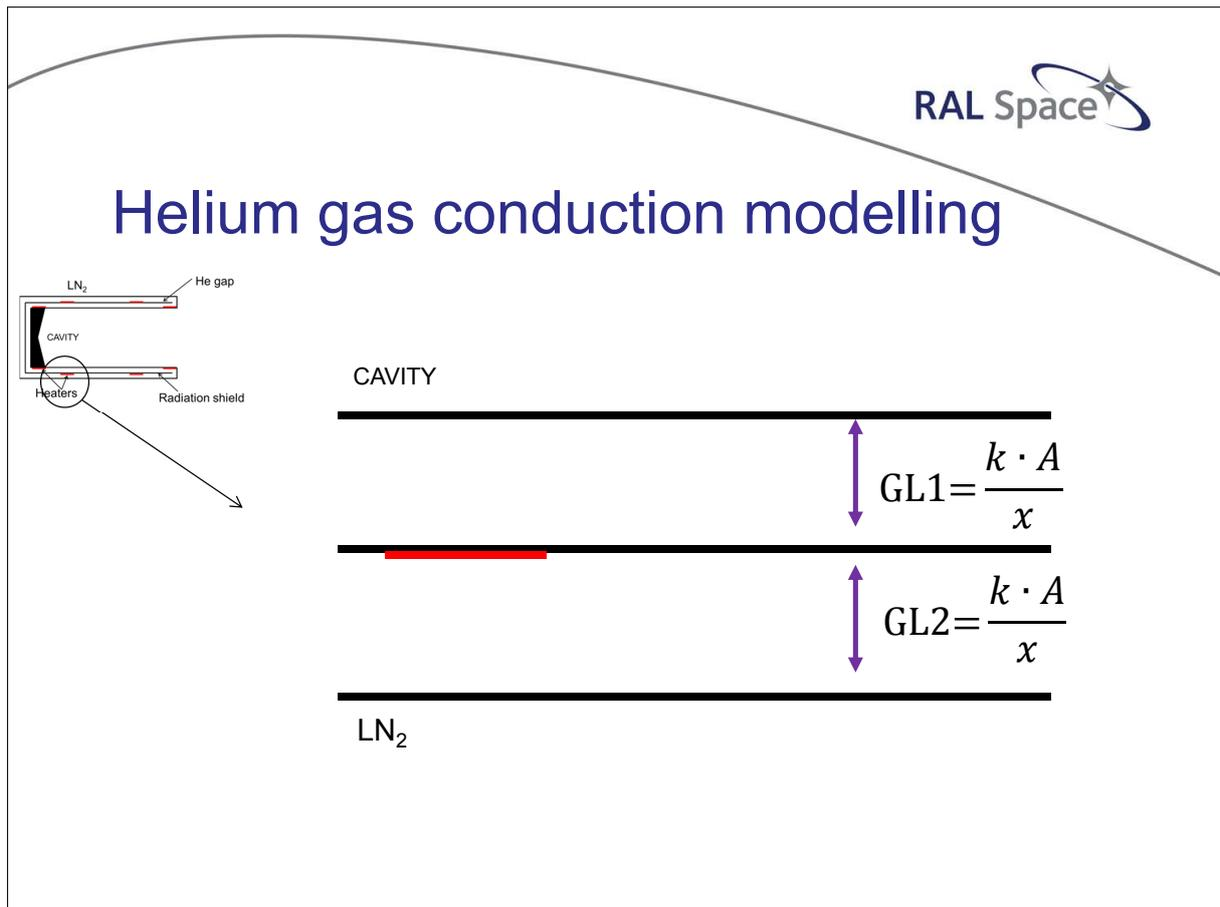
For the other conductive links in the thermal model, such as the bolted interfaces, I used the ESATAN Workbench to define a contact conductance. However, I did not define any geometry to be the helium, and so all the helium conduction modelling was done through the ESATAN file
