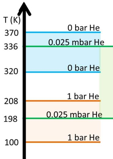
On a practical level it's easier to control the power input into heaters, than it is to control the pressure in a gas gap. So once I'd set up the model, I looked to see the smallest number of helium pressures I could use to control over the entire temperature range – given the 3 kW power limit.
