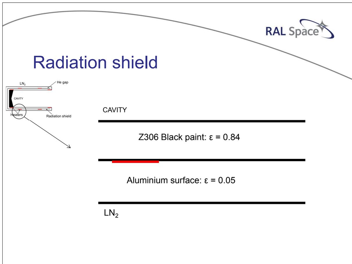
Since the main control heaters are on the radiation shield, we need to ensure that there is always a thermal link between the heated shield and the cavity, even when there is no helium in the gas gap. Conversely, on the other side of the shield, we want the thermal link between the cold liquid nitrogen and the shield to be dominated by the gas conduction.
