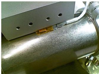
Temperature sensor of one motor housing
