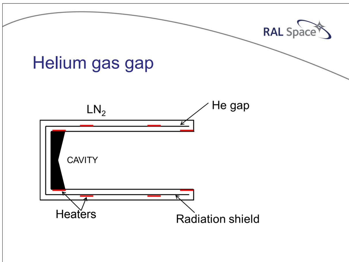
Helium's thermal conductivity changes with pressure, and so with 1 bar of He we get the maximum conductive link, with 0 bar, we get a vacuum and effectively no conductive link through the gas gap. At pressures in between we get varying conductance – hence the idea to operate the gap as a variable conductance gas gap heat switch.
