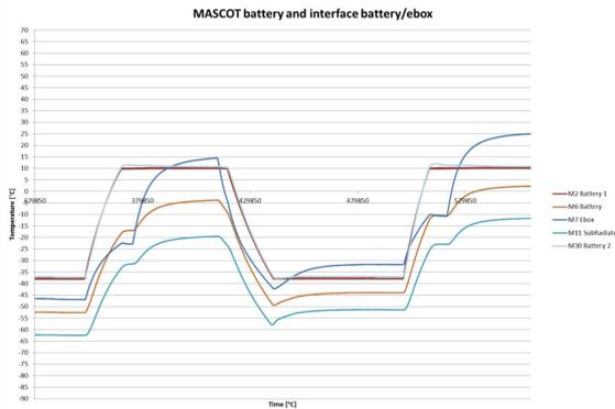
Different battery cells reach quite similar temperatures in all test phases.
