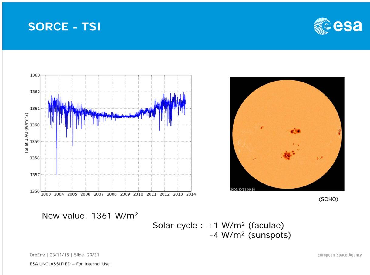
The Total Irradiance Monitor on NASA's Solar Radiation and Climate Experiment satellite measures the Total Solar Irradiance much more accurately and gives a new lower figure. This value is now accepted by climate scientists and is recommended in the latest report from the United Nations Intergovernmental Panel on Climate Change.
