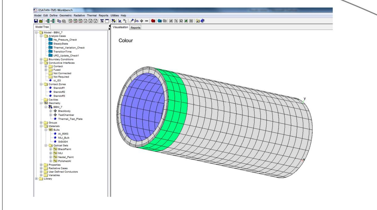
I've used this thermal model for the helium pressures and to optimise the heater distributions, and most recently to create the test predictions for the upcoming breadboard model tests.
