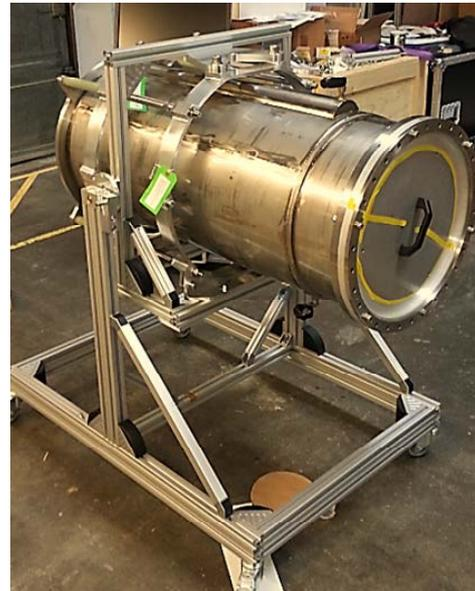
The breadboard model is a prototype of the blackbody that is being used to de-risk the design. It will provide loads of useful data to help me correlate the model and start on the more detailed CDR analysis.
