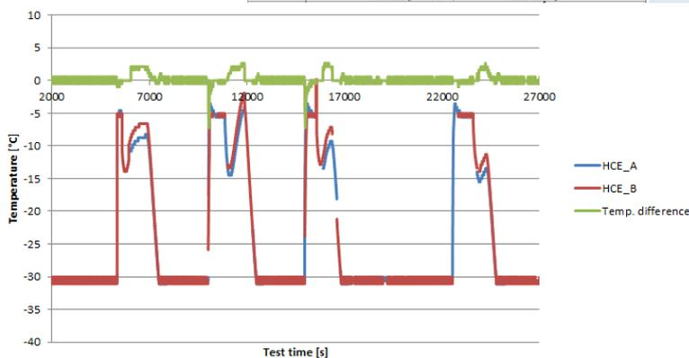
Regardless for the calibration fixed, temperature differences between the HY-2 sensors are present, moreover an anomalous long duration of pre-heating phases appeared.
