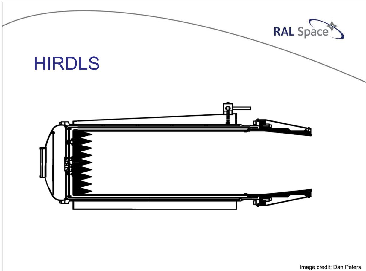
HIRDLS is an instrument that flew on the NASA Aura mission. The ground calibration target for this instrument covered the blackbody in a jacket of LN<sub>2</sub>, with a He gas gap between it and the cavity, and is the design that we have taken forward for the MTG calibration targets.
