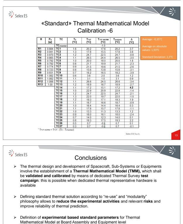
Issue of a (reduced) thermal models for different PCB board type (DC DC Converter, Control Board, Data Interface Board) to be used for what-if analysis and for reference for future projects
