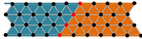
Guyan condensation to eliminate the detailed IF nodes
