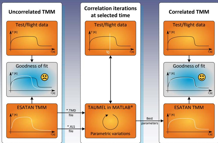
TAUMEL: Tool for AUtomatic Model correlation using Equation Linearization)
