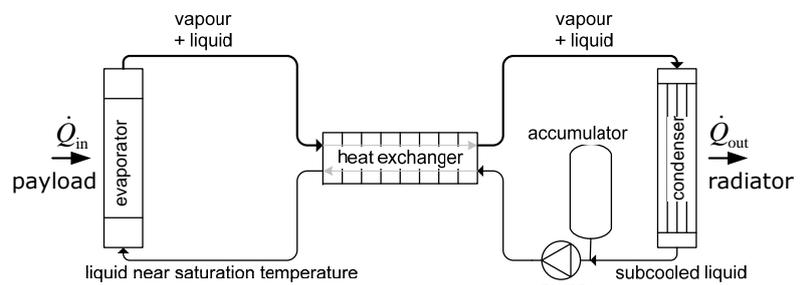
Schematic drawing of a 2 $\Phi$ -MPFL
