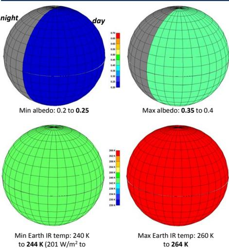
For the SRR and PDR, usual values of albedo and IR flux were used. Min albedo + min IR flux were cumulated with min Sun flux (winter), which is conservative. As the radiators can receive Earth flux only above the Polar regions, we legitimately wonder if our hypothesis were not too conservative, leading to oversize the FPA and FEE radiators
