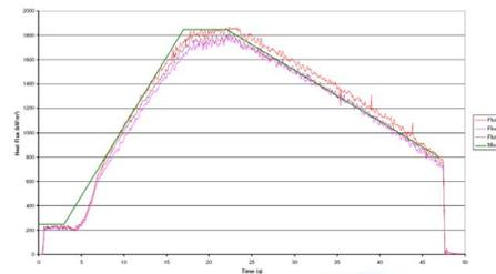
SIMOUN  $CO_2$  test conditions deliver conservative, flight-representative aerothermal conditions on a Flat Plate sample, in terms of cold wall heat flux, shear stress, local pressure evolutions.
