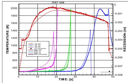
$$\alpha(H_a - H_w) + \epsilon\sigma(T_r^4 - T_w^4) + \dot{m}_s[H_g] + \dot{m}_c[H_c] = -\lambda \frac{\partial T}{\partial x}$$
