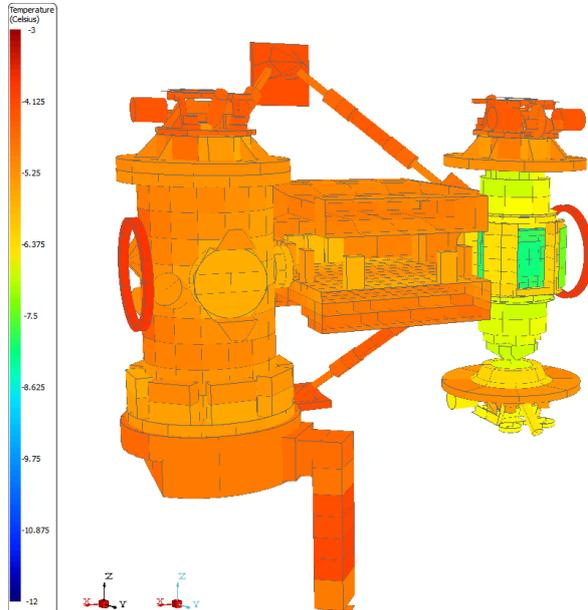
The temperature gain due to the boundary temperature oscillation (1mHz frequency) is calculated and plotted (in logarithmic scale) on the Geometrical Mathematical Model.
