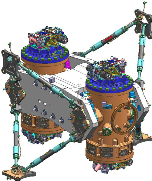
The LCA is composed by two Inertial Sensor Heads (ISH) separated by an optical bench. The whole assembly is connected to the LCA cage by means of 8 low conductance CFRP struts
