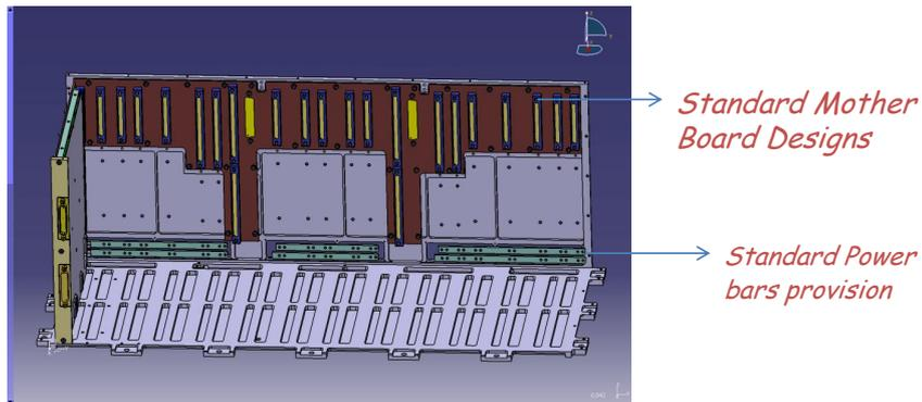
*Modular Architecture: Standard Mother Board Designs, with different configurations according to connectors layout*
