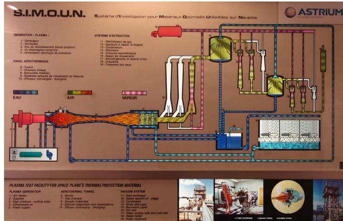
SIMOUN delivers a Mach 4, high enthalpy ( $H/RT_0 \sim 100$ ), low pressure ( $P_e \sim 0,1$  bar), air /  $CO_2$  flow. Uniform conditions can be obtained on Flat Plate 30 cm wide samples, possibly using a wedge. A Stagnation Point configuration is as well available.
