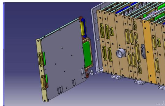
*Modular Architecture: The unit is assembled with Standard PCB Modulus design: the unit «connector wall» consist of the different PCB modulus front supports*
