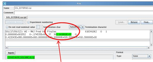
Via Optimus, the input parameters are changed as a variable. The user can choose a different probabilist law for each parameter.
