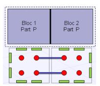
To sum up, user's task is reduced to interface resistivity definition. The rest of the geometry-based conductive model is computed automatically.
