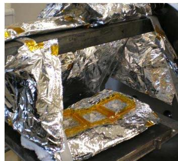
Plexiglas substrates placed in vacuum chamber
