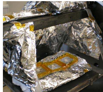
Plexiglas substrates placed in vacuum chamber
