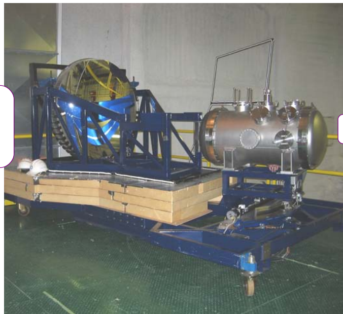
Spectrograph Structure with Main Mirror
