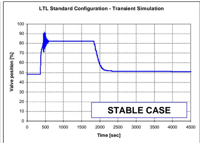
Heat variation:  $\pm 10$  kW (max injected power: 11.2 kW)
